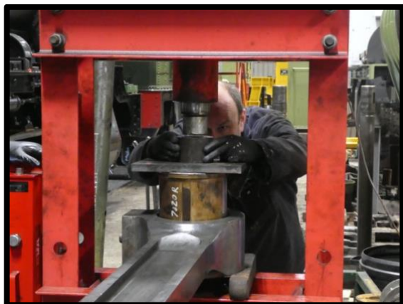
Mark lining up the big end bearing ready to be pressed back into the rod
